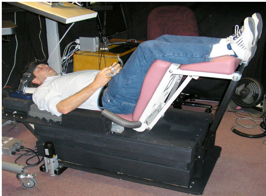
Figure 1. Ames' Three Degree-Of-Freedom Vibration Chair illustrating the experimental configuration.
