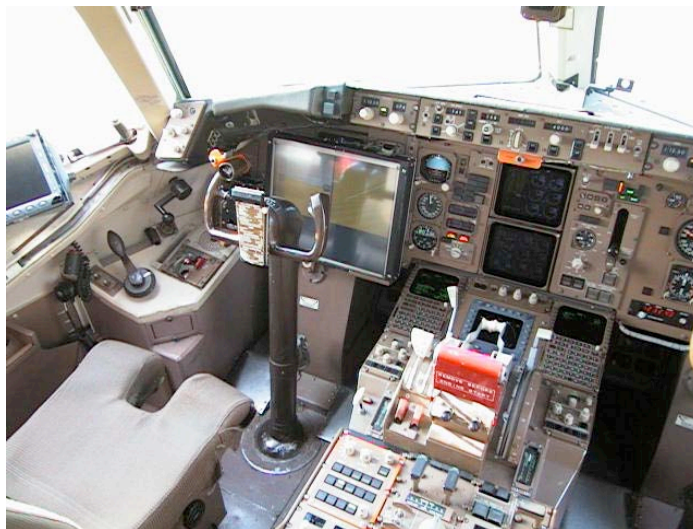
Figure 12. SVS in a NASA test aircraft.
