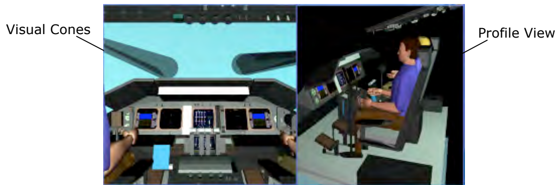
Figure 3. Runtime visualization of physical and anthropometric models carrying out procedures in the Jack™ environment. The left panel illustrates the view from the center of the cockpit and the right panel illustrates the left seat pilot's profile.
