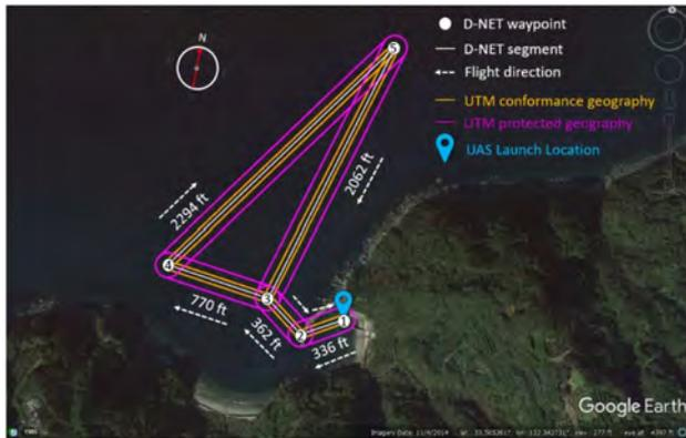
Fig. 11 UAV1 original flight plan and operation volumes.
