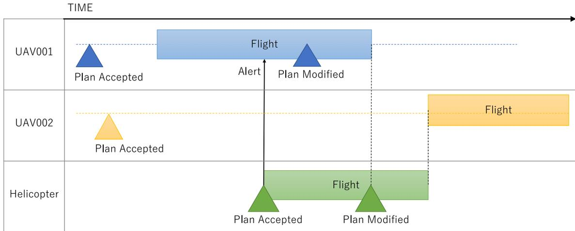
Fig. 5 Flight test operation timeline.
