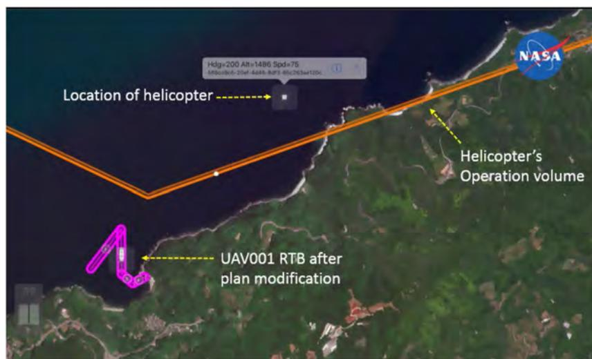
Fig. 14 Helicopter's operational volume, location, and UAV1 modified flight plan.
