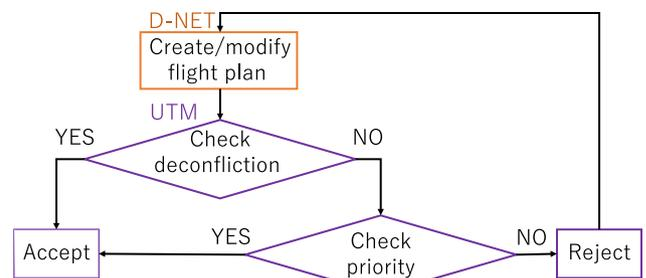
Fig. 6 Flight plan acceptance flow.
