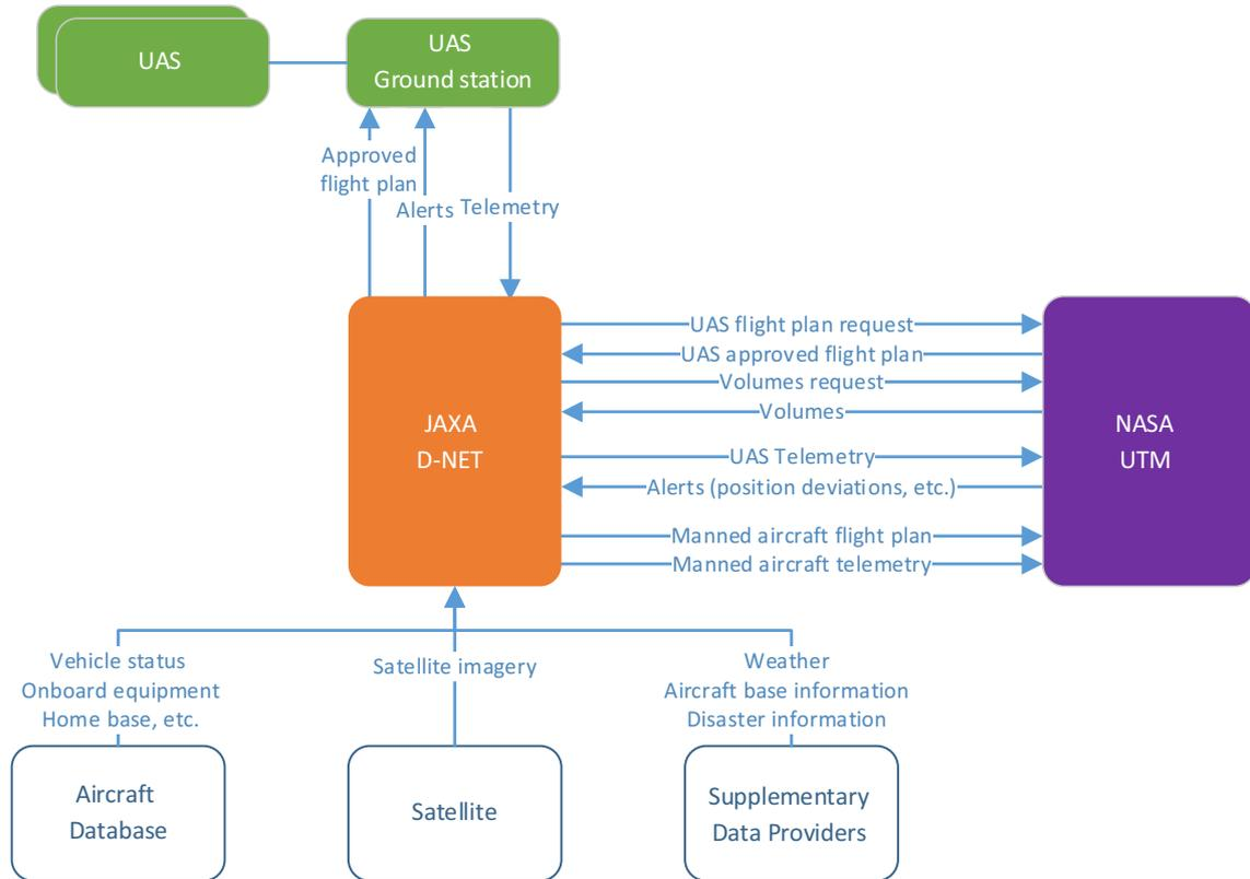
Fig. 3 D-NET/UTM interface architecture.
