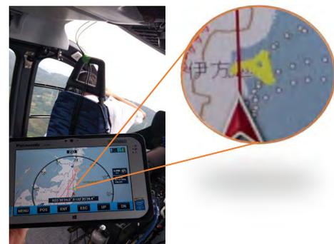
Fig. 12 Onboard D-NET portable system view. UAV area is shown in yellow, and the present helicopter position is shown by the red arrow.
