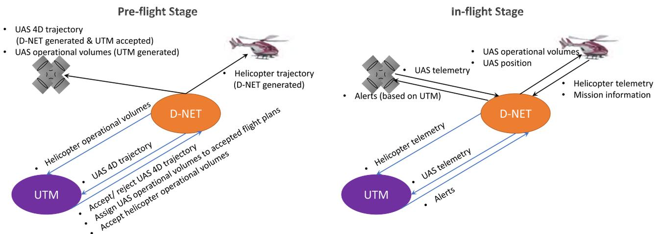
Fig. 2 D-NET/UTM conceptual interaction.
