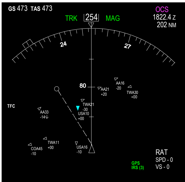
Figure 7. Using the route assessment tool (RAT) and showing a new SA 2 conflict along a potential path. Blue is depicted as bold white.
