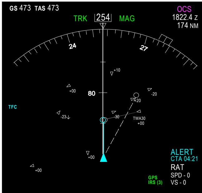
Figure 9. Using the RAT to find a clear path resolution to an SA 3 alert. Blue is depicted as bold white.
