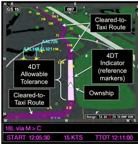
Fig. 2. Airport Moving Map (AMM) in the defined -tolerance display format with 4DT indicator (black reference lines in front of the ownship) and +/-405 ft allowable tolerance (light pink band).
