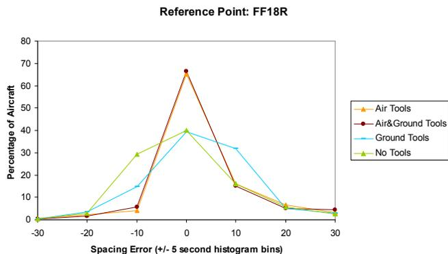
Figure 4. Spacing accuracy at the runway 18R final approach fix.
