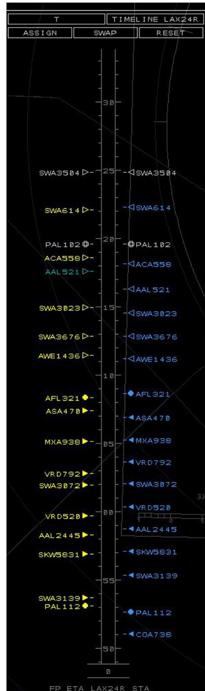
**Fig. 3** LAX24R schedule timeline with aircraft wake category symbols. Estimated arrival times are shown on the left; the right side shows scheduled times of arrival, with the wake category symbols filled in for aircraft with ‘frozen’ scheduled times.
