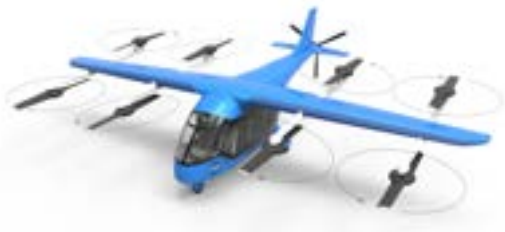
Fig. 1. NASA RVLTL Lift-Plus-Cruise conceptual model
