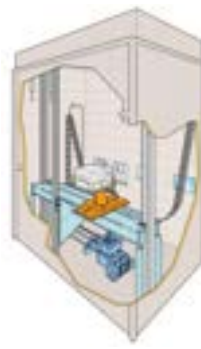
Fig. 2. Drawing with layout of the Vertical Motion Simulator
