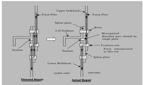
Figure 3. The repair to the aft pressure bulkhead as specified in the repair instructions (at left), and repair as actually carried out (on right). Note gap of doubler plate between top two rivets. Source: Terada and Kobayashi (2006).
