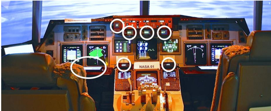
Fig. 1. Flight deck in RCO with Collaboration Tools condition. The six CRM indicators are mounted adjacent to their corresponding instrument panel. Captain’s EFB is circled to the left.
