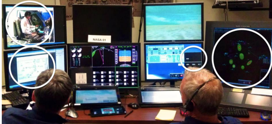
Fig. 2. In RCO with Collaboration Tools condition, the traffic and weather sector map (circled, far right) and the charts and approach plates display (circled, mid-left) can be shared with the Captain, who is shown in the Video Feed (circled, upper left). Ground CRM indicators are to the left of the traffic and weather sector map. The ground operator shown is in CT training.
