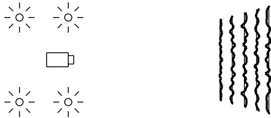
Figure 2: Range recovery of planar surfaces; a simulated camera looks from left-to-right at a planar surface illuminated by four different lamps. Heavy lines show the reconstructed range. The range of depths of the test surfaces corresponds to the range used in the training set.
