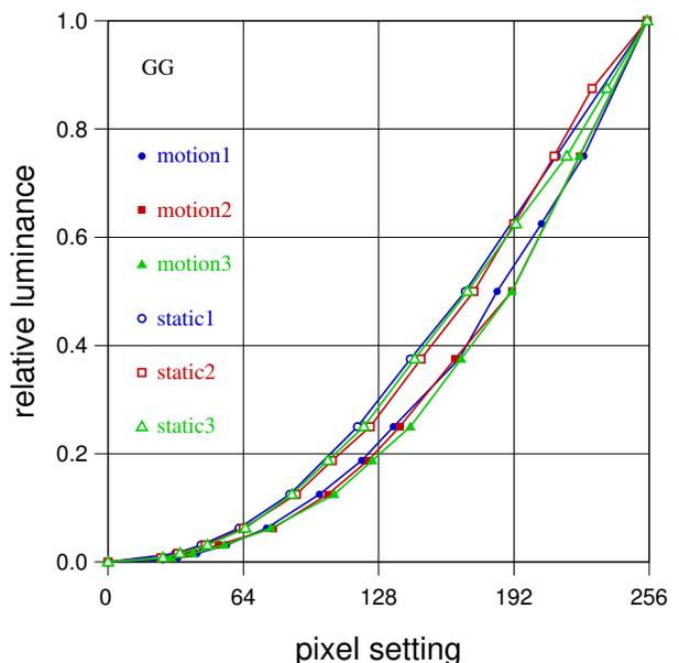
Figure 3: Gamma functions estimated using the static method (filled symbols) and the motion method (open symbols), for subject JBM (upper panel) and GG (lower panel).
