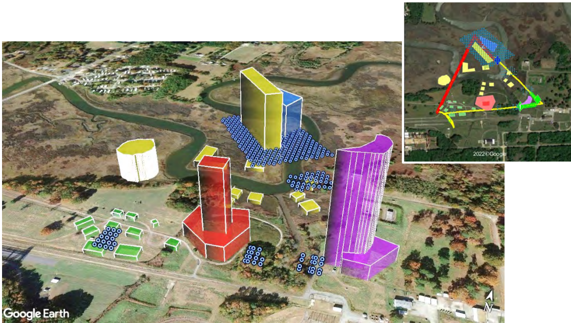
Fig. 3.2-1. Collision and population overflight virtual hazards. Population is shown as blue circles and structures as colored geometries in 3D (foreground) and 2D (inset).
