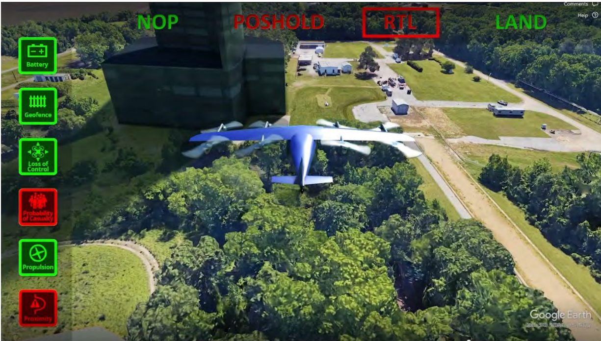
Fig. 3.3-1. Example of prioritization of the most urgent action with two safety alerts to direct the most urgent flight command at one moment in flight 102. Collision with a virtual building is threatened and vertical descent to land would threaten the underlying ground population. The monitor/assess/mitigate architecture selected RTL, diverting the aircraft to land at an alternate safe landing site. From [44].
