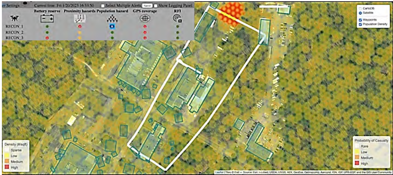
Fig. 2.2.3-3. Image of SDSP-CD display interface showing underlying population density that gives rise to the hazard alert highlighted in Fig. 2.2.3-2. Population density (yellow hexagons) and a probability of casualty heat map (red hexagons) is overlaid on a map of buildings (blue polygons). From [44]. (NASA image)
