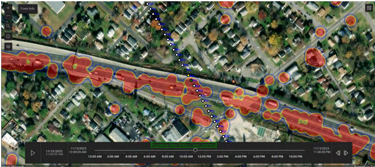
Fig. A.1-2. Closeup view of flight segment over city of Hampton, VA. In this example, colored dots indicate locations along the flight path where the casualty risk is estimated/predicted to be the higher due to elevated population presence below and near the flight, e.g., on the highway and streets.
