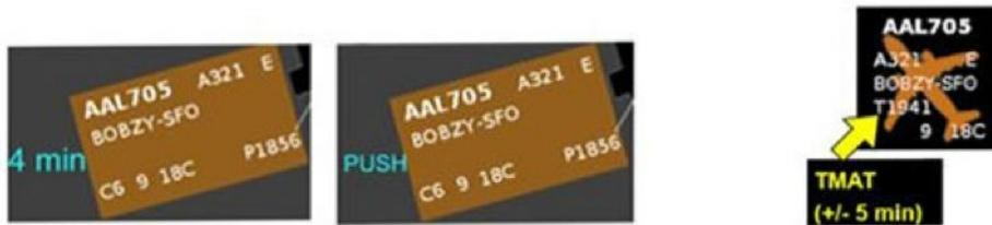
**Fig. 3.** Flight strips for aircraft in both metering conditions: (left) at gate showing gate hold advisory countdown (“4 min”) to the TOBT (Target Off-Block Time); (middle) at which time “PUSH” is indicated; (right) after pushback with TMAT (Target Movement Area entry Time) showing “1941” for arrival at the spot.
