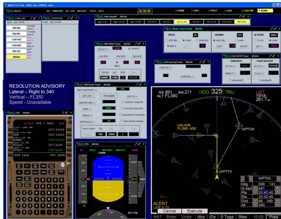
Figure 8. Example MACS station equipped with CDTI and agent support controlling several (here 6) aircraft
