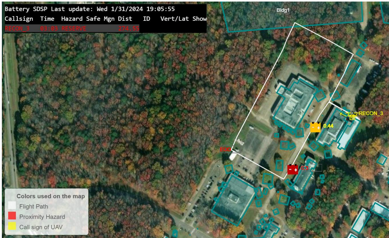
Fig. 4 Image of the SDSP-CD interactive map showing the battery reserve service for a vehicle’s proposed flight path (in this example, the vehicle is flying clockwise on the route). The yellow battery icon indicates where the vehicle’s battery will reach the reserve-limit that was set by the user and the red battery icon indicates where the vehicle’s battery will drop below that threshold. The red EOD marker indicates that, with the current flight path, the vehicle would land with a battery reserve below the user’s set threshold. The information table pop-up is located in the top left and can be moved by the user to any desired place on the interactive map. (NASA image)
