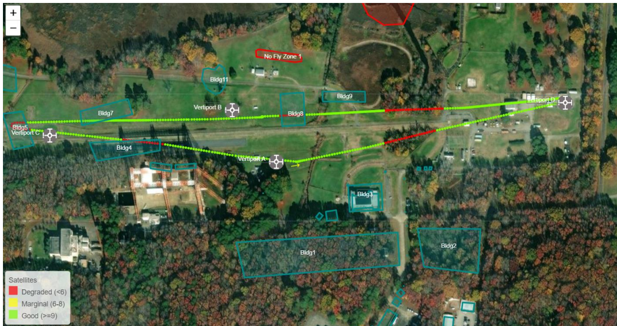
Fig. 3 Image of the SDSP-CD interface showing a proposed flight path with the GPS signal strength service shown on the interactive map. When the GPS service is selected, the route is illustrated as a series of dots, with each dot representing a point along the route. Each dot is color-coded to map to the three GPS signal strength designations (i.e., good, marginal, and degraded). A legend at the bottom left of the map provides users with the meaning of each signal strength designation. (NASA image)
