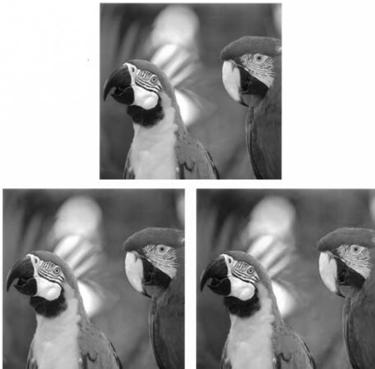
Fig. 17. Original image (top) and compressed with perceptually lossless DWT quantization matrix (bottom left) and twice that matrix (bottom right). Image dimensions are 256 \times 256 pixels. Quantization matrix is designed for a viewing distance of 23 in.
