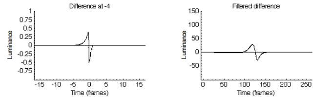
**Figure 11.** Difference between an ideal edge and the apparent edge (left), and the filtered difference (right). The results are for an edge that has been shifted in order to minimize the pooled error between the two functions.
