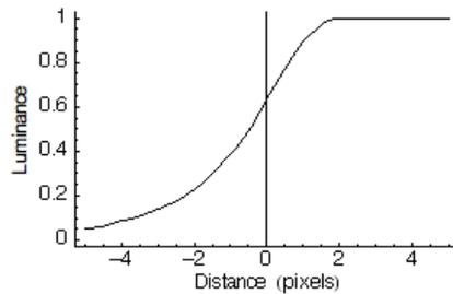
**Figure 9.** The apparent edge function for an exponential transition function with a time constant of  $\tau = 1$  frame (Figure 1), and a speed of  $r = 2$  pixels/frame.
