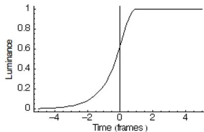
**Figure 10.** The temporal edge blur for an exponential transition function with a time constant of  $\tau = 1$  frame (Figure 1).
