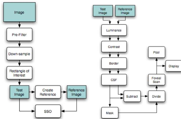
**Figure 3. A. Preprocessing of the captured display image and creation of the reference image. B. Application of Spatial Standard Observer to mura measurement.**
