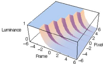
**Figure 6. The edge function for an edge speed of  $r = 2$  pixels/frame and an exponential transition function with a time constant of  $\tau = 1$  frame (Figure 5).**
