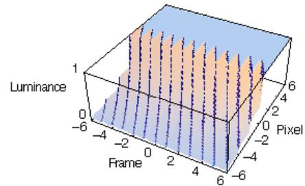
**Figure 7. Stabilized edge function for an exponential transition function with a time constant of  $\tau = 1$  frame (Figure 1).**
