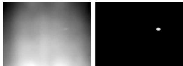
**Figure 4. Example of SSO mura measurement. The left image is a capture of a 17 LCD panel. The right image shows the SSO output image, thresholded at 2 JND. The peak value is 4.1 JND.**
